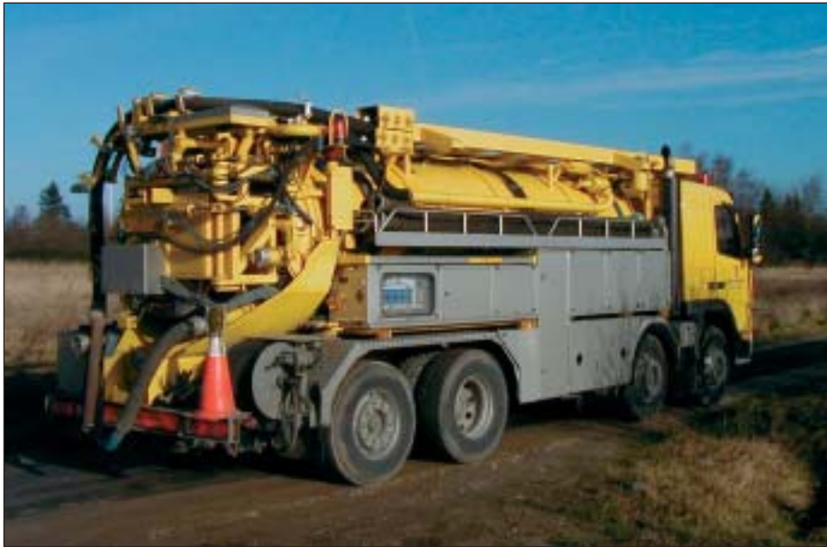
High-pressure flushing vehicle.
