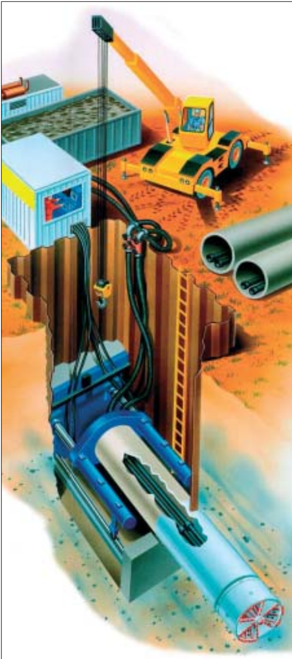
Schematic illustration of microtunnelling
