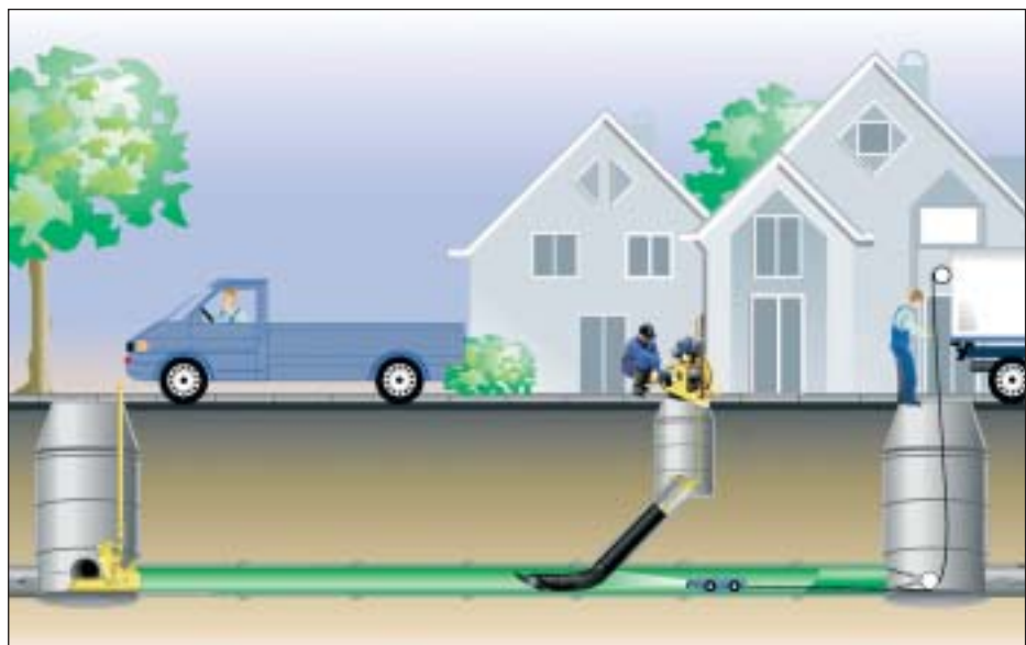
Close-fit lining and subsequent lateral installation.
